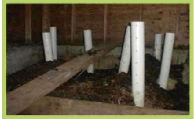
*Perforated PVC pipes for aeration.*
